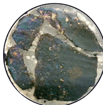
Fig. 2: Chalcopyrite cut in epoxy resin.
